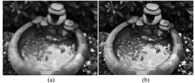
Fig. 3. Example of reconstructed images with different sparsities. (a) Reconstructed image with sparsity = 1. (b) Reconstructed image with sparsity = 6.
